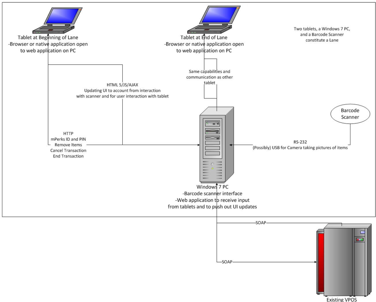
Figure 9: System Architecture Diagram
