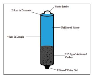
Water Filtration Design Project: Student Water Filtration System Design
