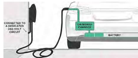
On-board Charger in an Electric Vehicle
