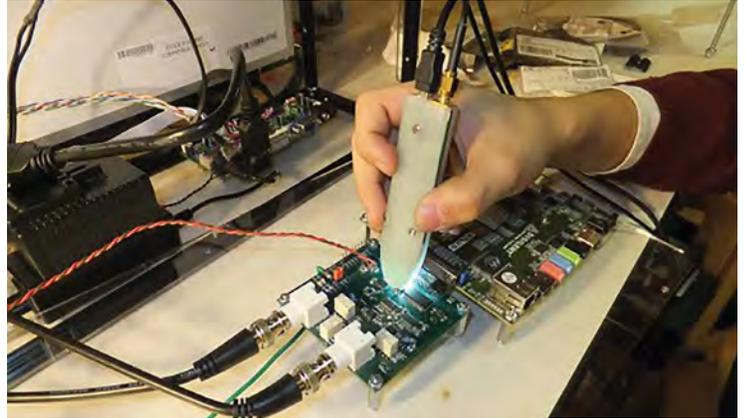
bandwidth, high input impedance, relatively large differential input range, BNC connector output to interface to an oscilloscope and Electrostatic Discharge (ESD) protection system. While these types of probes are typically quite expensive (costing roughly \$5000 USD), we aim to produce this probe for less than \$500 USD.
