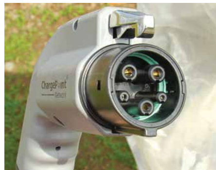
SAE J1772-2009 Electric Vehicle Connector
